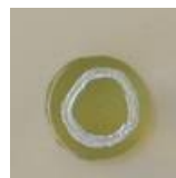
The screed is dry! (RH<85%)
